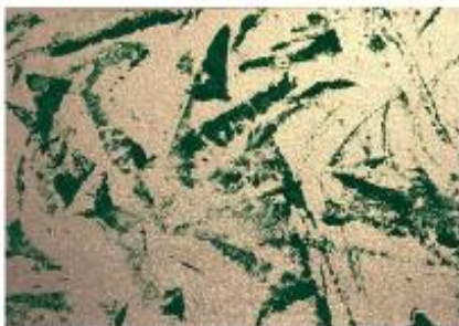
Base Coat: Silver Sparkle 4194 (10-100 µm) Top Coat: Green Decorative
