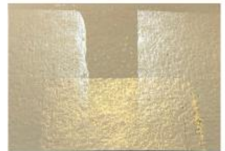
Base Coat: White Decorative Top Coat: Iridescent Gold 4195 & Blue 4197 (10-60 µm)
