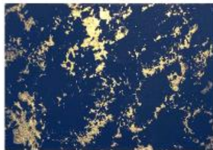
Base Coat: Blue Decorative Top Coat: Iridescent Gold 4195 (10-60 µm)
