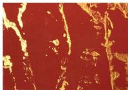
Base Coat: Red Decorative Top Coat: Sparkle Gold 4144 (10-100 µm)
